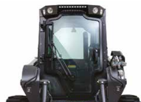
FRONT DEMOLITION DOOR
